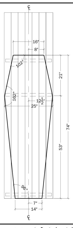
Flip the boards over so the temp cleats are facing down. Layout the coffin and cut out (Cut through the cleats as well)
