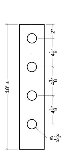
I used a 1-3/8"Ø closet rod dowel from Lowes for the handles.
