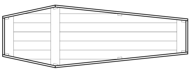
When attaching the vertical cleats, I would shoot one staple in then square it up and downwith the bottom. This made running the 2nd and 3rd layer much easier
